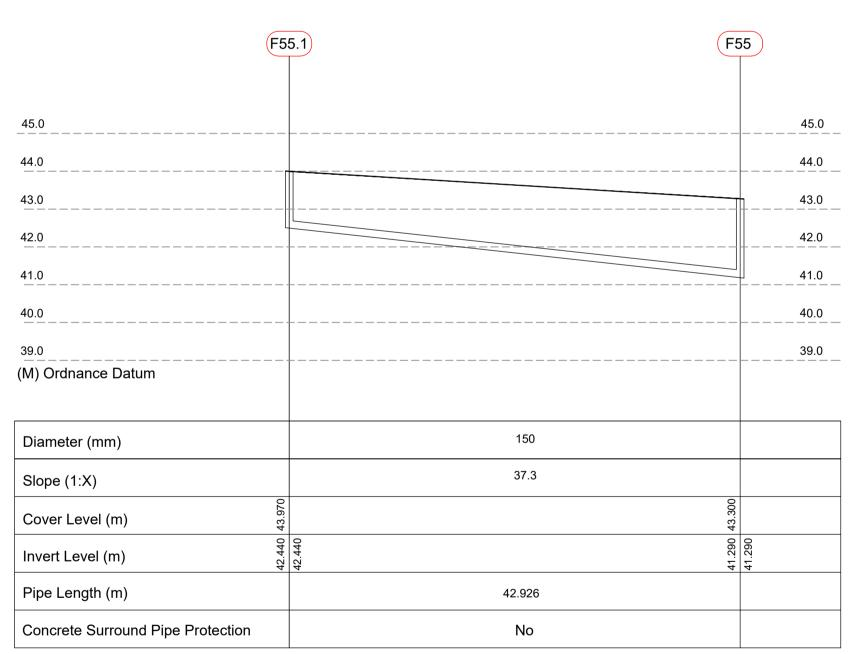
FOUL SEWER LONGSECTION F55.1 TO F55 HORIZONTAL SCALE 1:500
