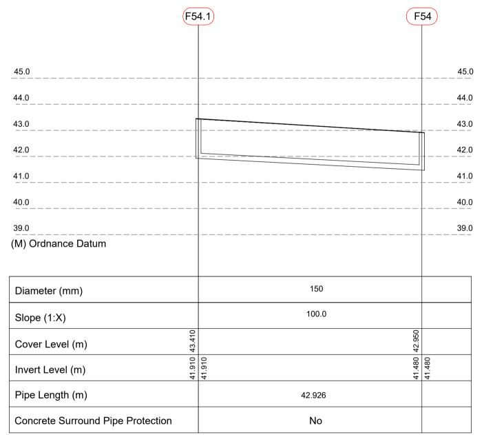
FOUL SEWER LONGSECTION F54.1 TO F54 HORIZONTAL SCALE 1:500 VERTICAL SCALE 1:100
