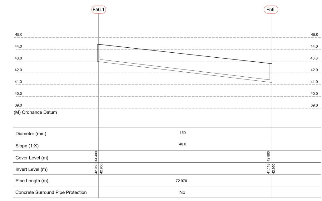
FOUL SEWER LONGSECTION F56.1 TO F56 HORIZONTAL SCALE 1:500 VERTICAL SCALE 1:100
